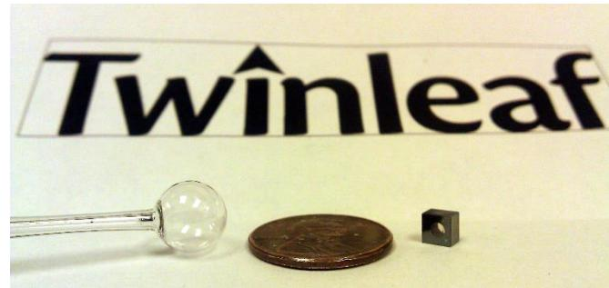
$^{129}\text{Xe}$  wall  $T_2 = 100 \text{ s!}$  in anodically bonded cell
