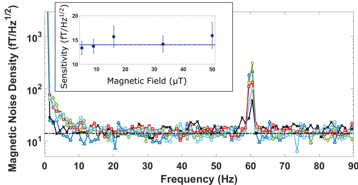
Subtracting two magnetometer frequencies and using fitting times of 5 ms, we find a differential field sensitivity of  $14.7 \Delta f/\text{Hz}^{1/2}$ . The all-optical gradiometer shows no loss of sensitivity with bias fields outside the SERF regime, due to spin-exchange relaxation suppression from high Rb polarization. We also find a common mode rejection ratio of  $10^4$ .
