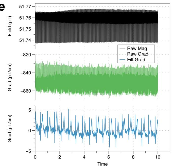
This work informed a next-gen gradiometer with a 3 cm baseline. USB powered and ran from a laptop, we detect heartbeats in a noisy environment in Earth's field.
