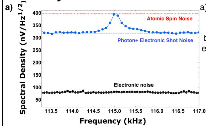
a) Spin noise spectrum for unpolarized spin ensemble at  $B_z = 16 \mu\text{T}$ , along with electronic and photon noise.
